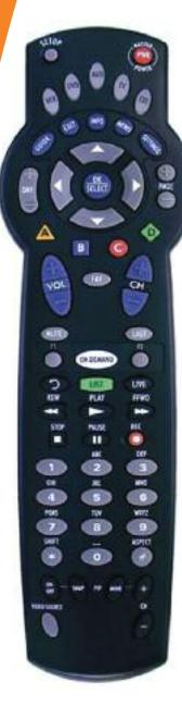
These are your power buttons. Just press the button for the device you'd like to turn on or off. Or, use the **All On** button for multiple devices. Now you can record, play, fastforward, rewind, stop, and pause using your ON DEMAND\* & DVR buttons.
